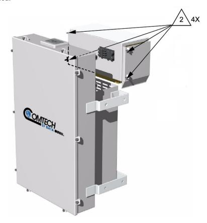
Figure C-1. Remove/Replace the HPOD Power Supply
